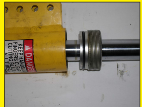
Carefully withdraw ram and end cap
