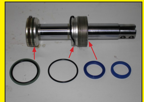
Remove and replace end cap seal reassembly is the reversal of removal
