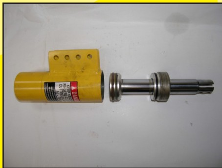
Only remove fully if piston seals are to be replaced also
