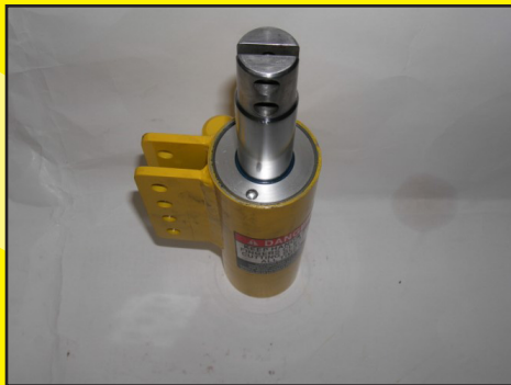
Identify end cap and holes to remove it
