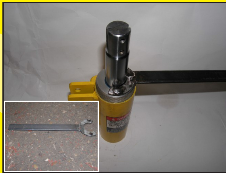
Using suitable tool unscrew end of cap in an anti-clockwise direction
